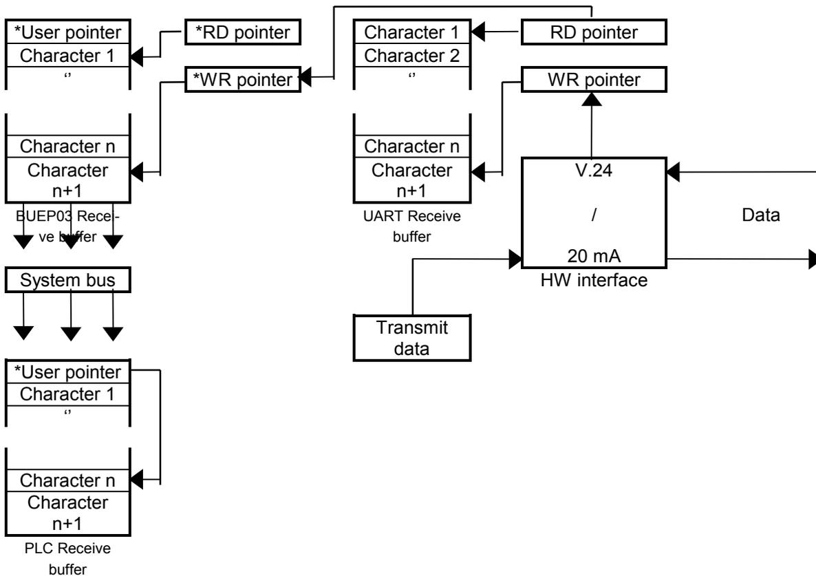
Fig.. 7-5 BUEP03E — Data exchange between Receive buffers
