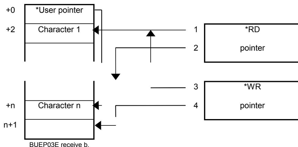
1+3 : RD and WR pointers after Reset Receive Buffer has been selected
