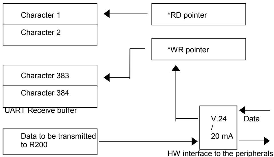
Fig. 7-3 UART Receive buffer
