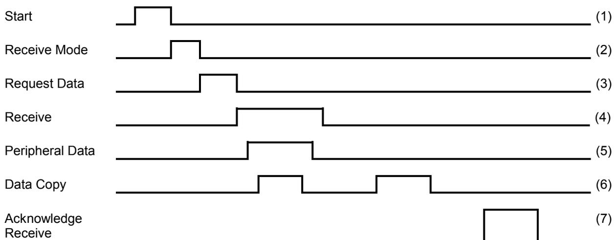
Fig. 7-7 BUEP03E — Chronological sequence of a single communication
